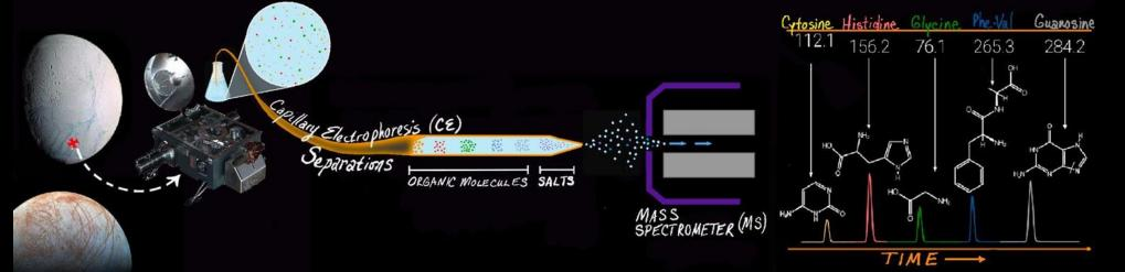
CE-MS's ability to deal with high levels of salts while allowing detection of a wide range of organics at parts-per-billion concentrations demonstrates that CE-MS is uniquely suited for detecting signs of life in future missions to ocean worlds.
